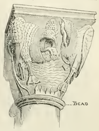
Bead as used beneath a capital.—Abbey-church of Vézelay, Yonne, France; 11th century. From Viollet-le-Duc's "Dict. de l'Architecture."
